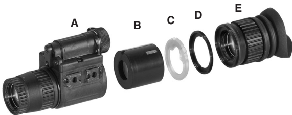
Figure 6-3 Maintenance/Replacement of the tube in the NVM-14
