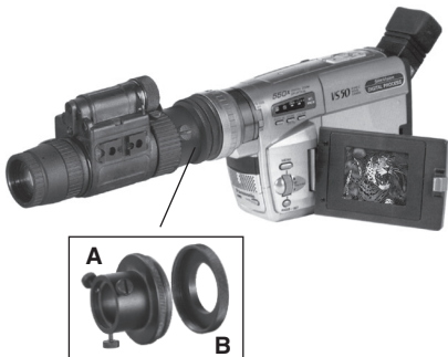
Figure 3-8 Mounting Camcorder to the ATN NVM-14
