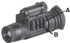
Figure 3-6 Mounting the Picatinny Adapter to the ATN NVM-14
