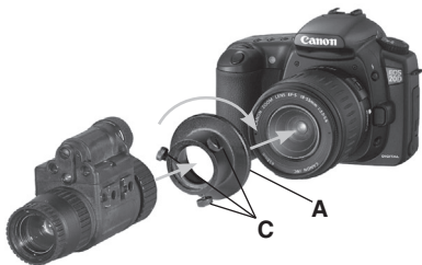
Figure 3-7 Mounting Camera to the ATN NVM-14
