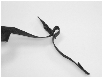
Figure 6-2 Lacing the Sliding Bar Buckle
