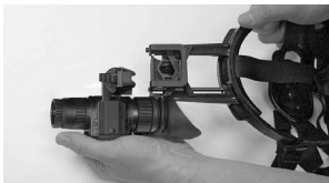
Figure 3-10 Attaching ATN NVM-14 to PVS-7 Headmount
